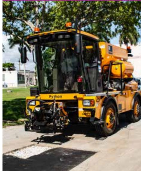
The Python 5000 Asphalt Pothole Patching Machine
